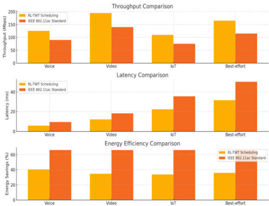
Fig.6. Cross-Traffic Performance Comparison: RL vs. IEEE 802.11ac
