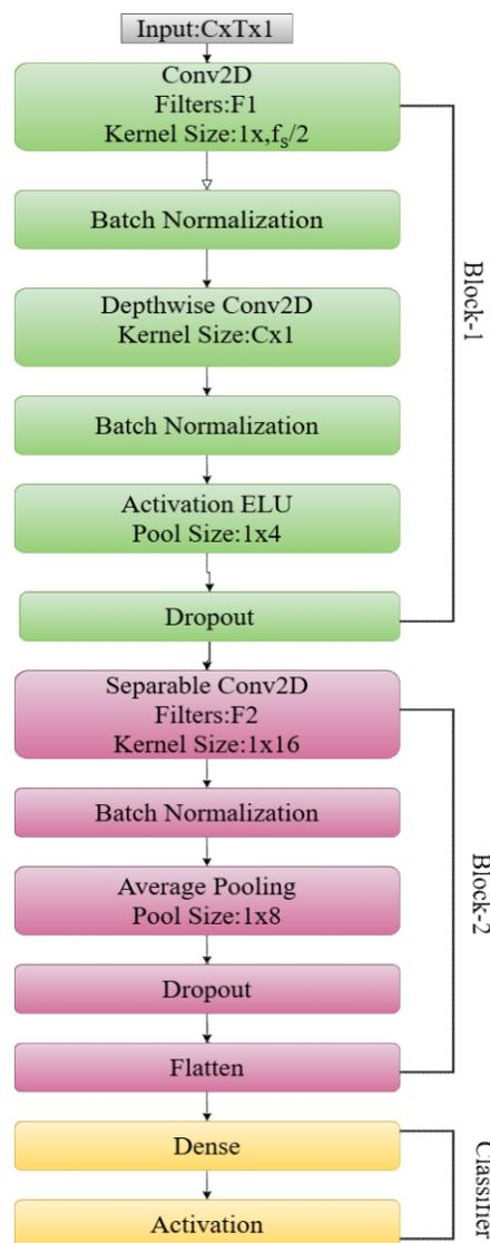
**Fig 4: Architecture of the standard EEGNet**
