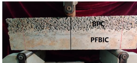
Figure 5. Three-point bending test specimens and experimental method.
