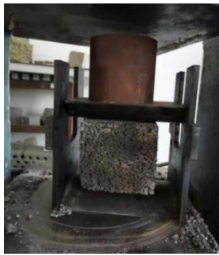
Figure 4. Composite specimen splitting tensile test.
