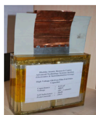
0.15 µF, 40KV, 20nH Flat-format Capacitor
