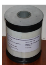
4uF, 10KV, 20nH Hollow Cylindrical Capacitor
