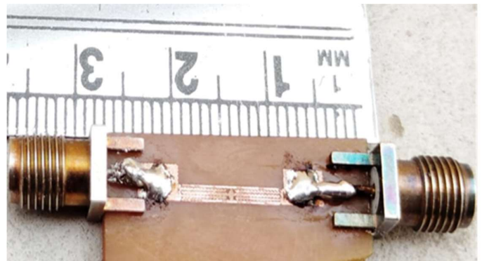
Fig. 9. Photograph of fabricated proposed filter
