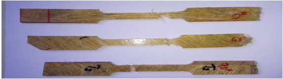
Fig.2 Failure tensile test specimen of Sisal fiber reinforced epoxy composites
