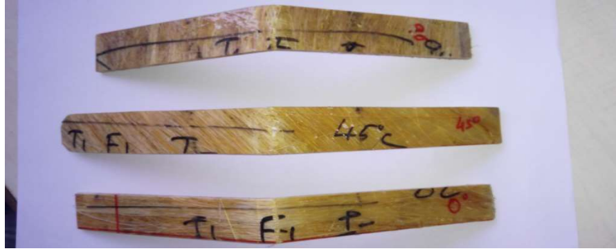
Fig. 6 Failure specimen of flexural test specimen
