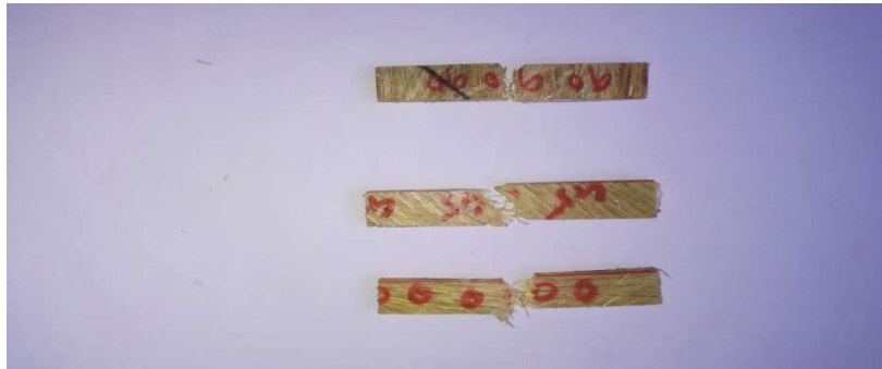
Fig. 7 Failure specimen of impact test specimen
