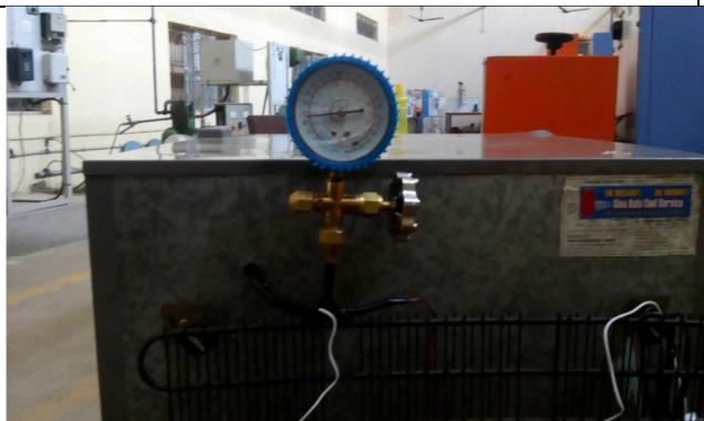
Figure 4. Rear view of mini refrigerator with copper capillary tube
