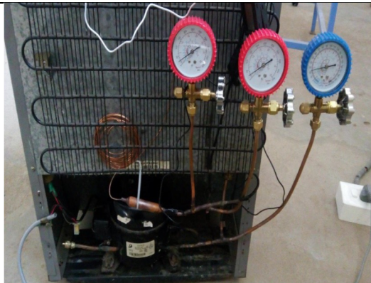
Figure 4. Rear view of mini refrigerator with copper capillary tube
