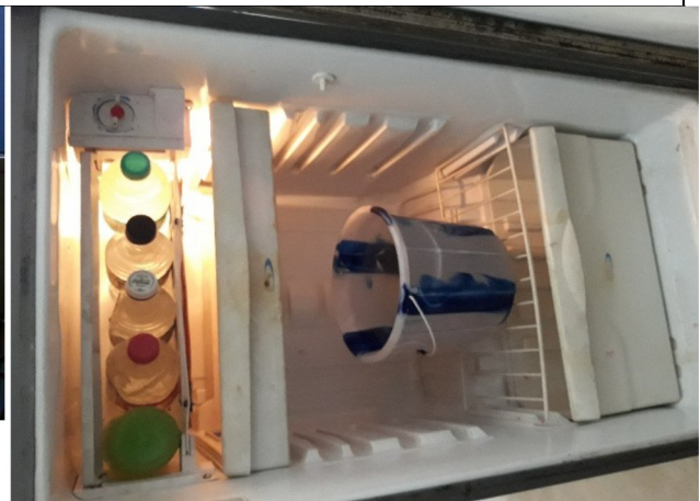
Figure 7. Inner view of mini refrigerator loaded with 10 kg of water
