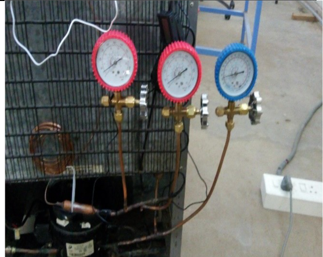
Figure 3. Rear view of mini refrigerator with high pressure and low pressure gauge
