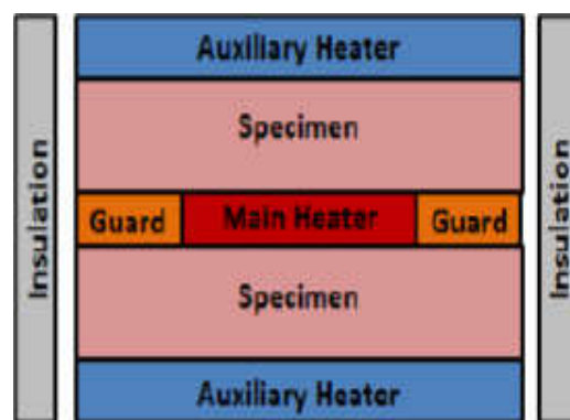
Figure 3. Schematic of Guarded Hot Plate Method
