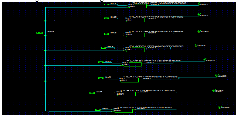
Fig.5: Schematic diagram of 8 Bit Multiport Register File in DSCH 3.9
