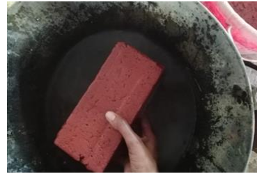
Fig. 3.2 Water absorption test
