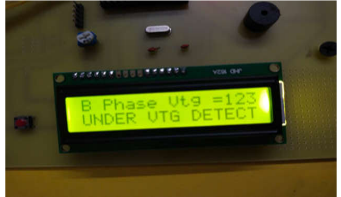
Figure 4: B-Phase Under Voltage Detected
