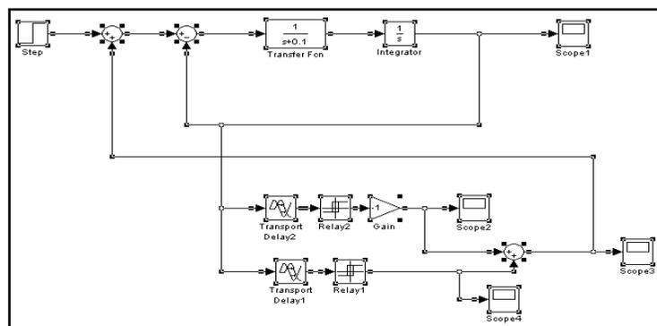
Figure 4.2: Simulation Diagram of Dead Beat System with pulse signal
