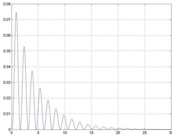
Figure 9.1(c). The mean square error of the output response between higher order system and reduced second order system of example 9.1.1
