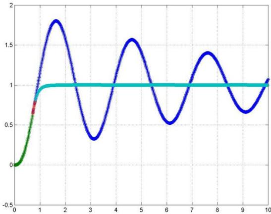
Figure 9.1 (a). Dead beat response of example 9.1.1 using same pulse parameters used in reduced second order system of figure 9.1(b)
