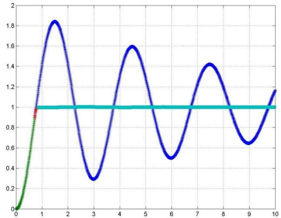
Figure 9.1 (b) Deadbeat response of example 9.1.1 used in reduced second order system of figure 9.1 (a)
