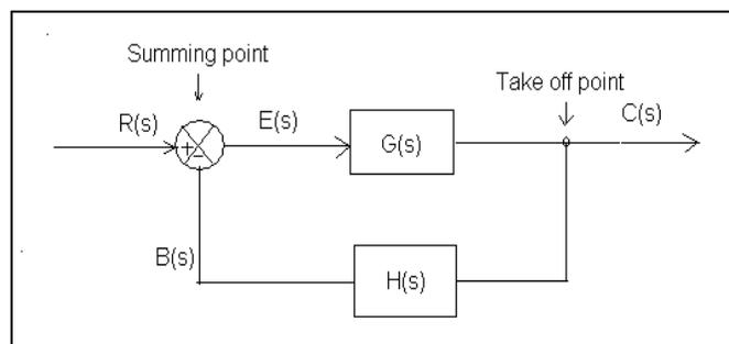
Figure 4.1: The input-output behavior of closed loop linear continuous system
