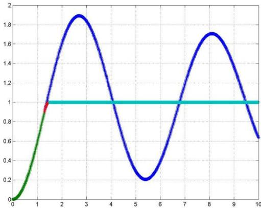
Figure 9.2 (b) Deadbeat response of reduced second order system of figure 9.2 (a)
