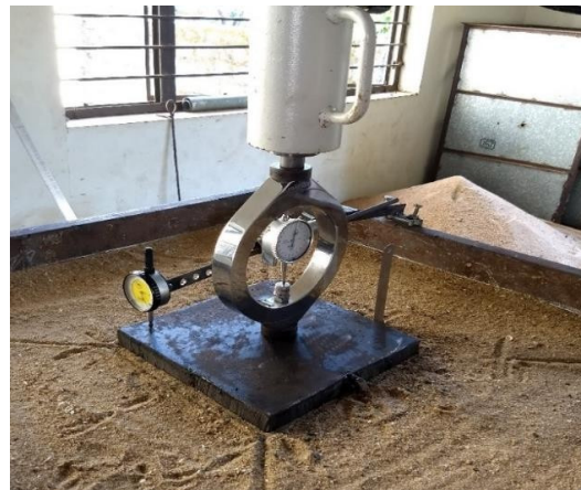
Fig -5: Axial loading setup
