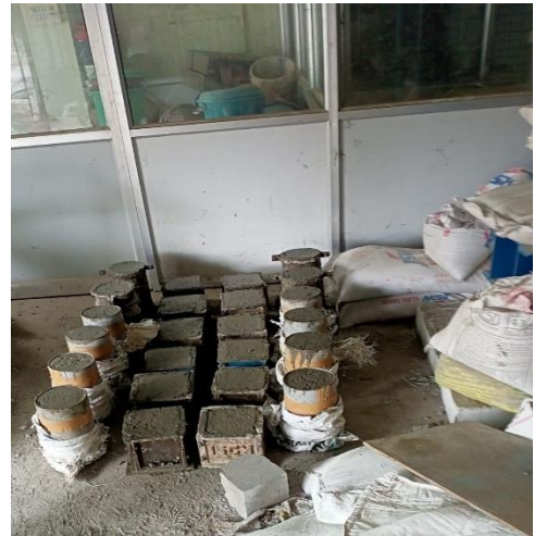
Fig.1: Preparation of Concrete block using casting method
