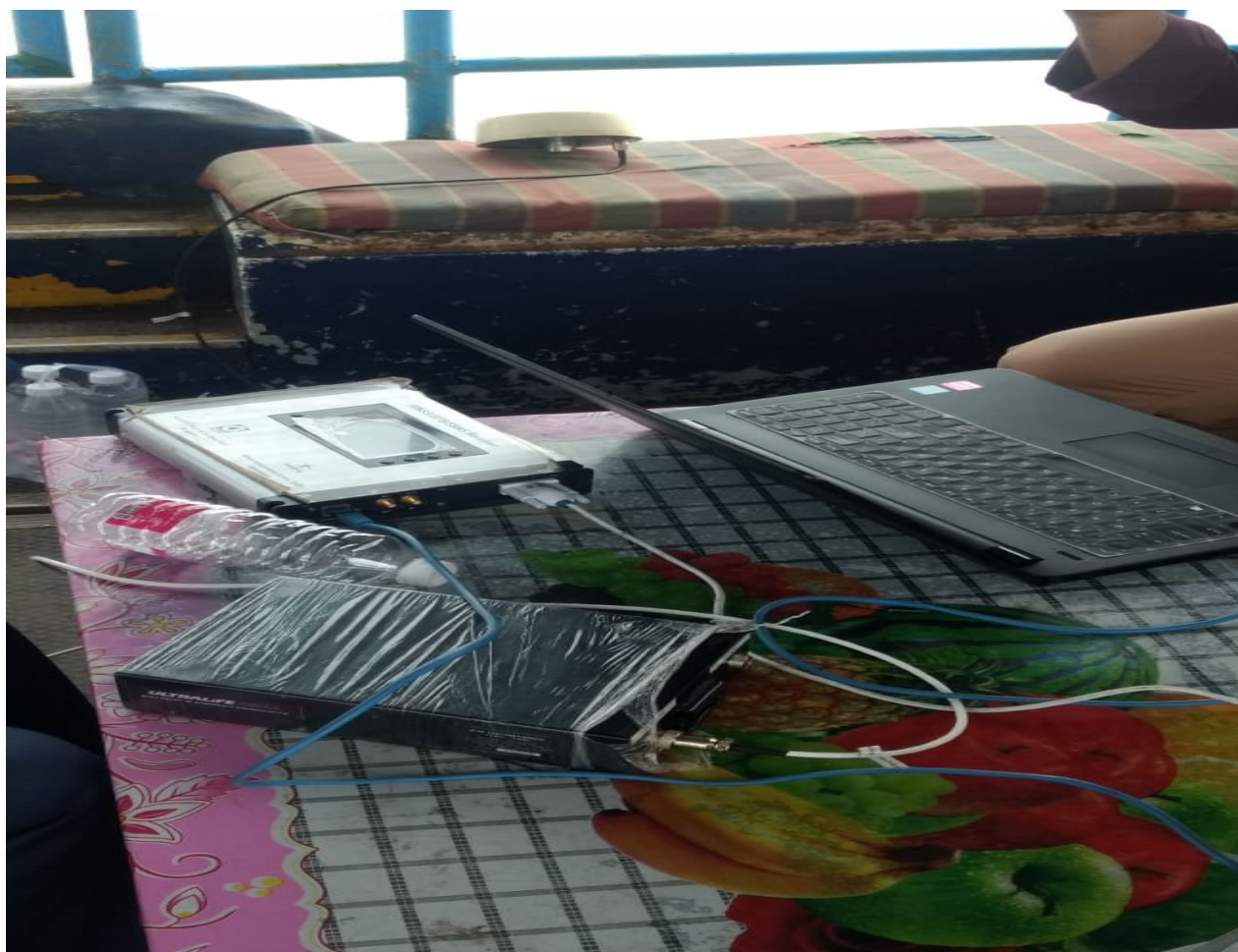
Figure.4. Experimental set-up of NavIC receiver in boat.
