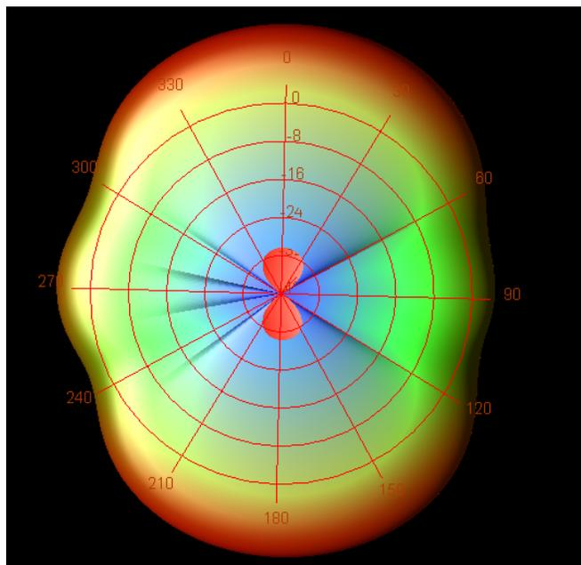
Fig. 6: Simulated 2D radiation pattern at 5.32 GHz
