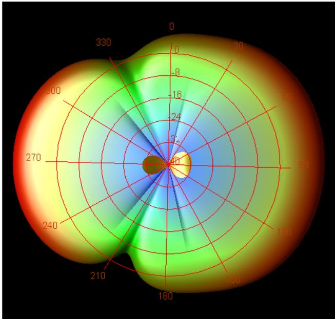
Fig. 7: Simulated 2D radiation pattern at 5.57 GHz
