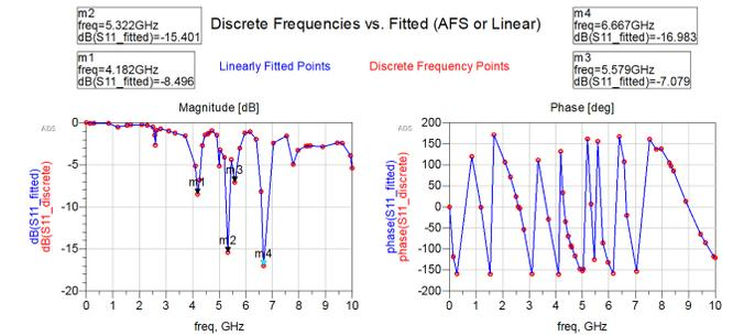
Fig. 2: Simulated return loss ( $S_{11}$ ) vs frequency
