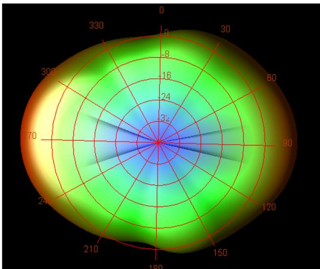
Fig. 8: Simulated 2D radiation pattern at 6.66 GHz
