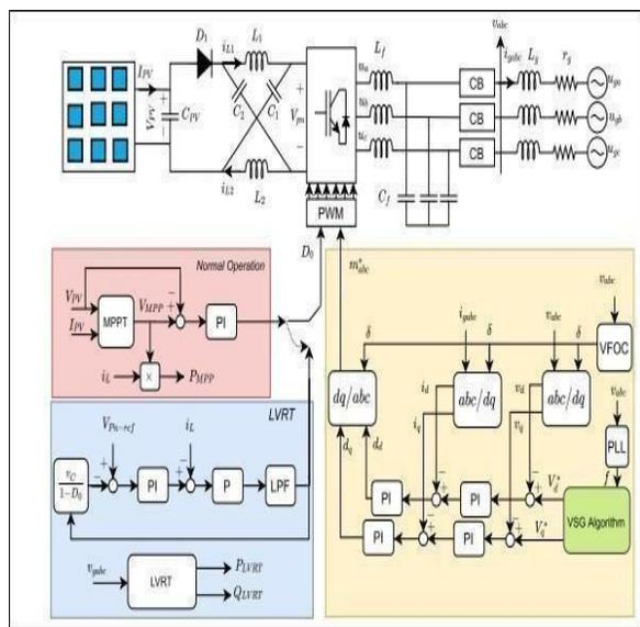
**Fig.1 Block diagram of Z-source virtual synchronous generator**
