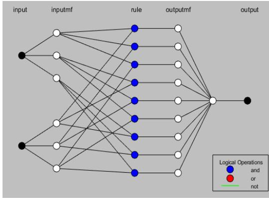
**Fig. 3 Structure of ANFIS Controller**
