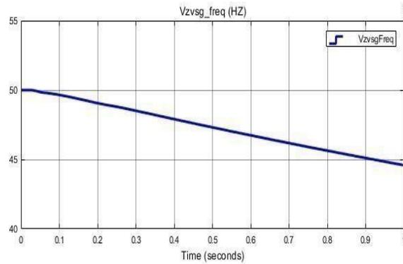
**Fig. 4 Frequency at ZVSG side**
