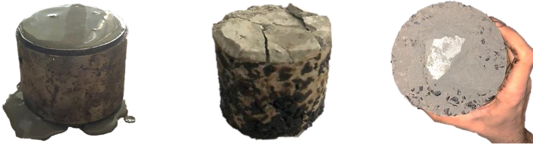
Figure.17 Grout with higher water content (w/c ratio = 0.6) showed good penetration but lacked strength.
