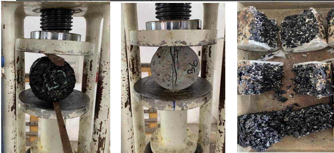
Figure.22 (a) Samples placed horizontally for testing (b) Failure of specimen observed as a split in the middle (c) Samples deformation after indirect tensile strength test.
