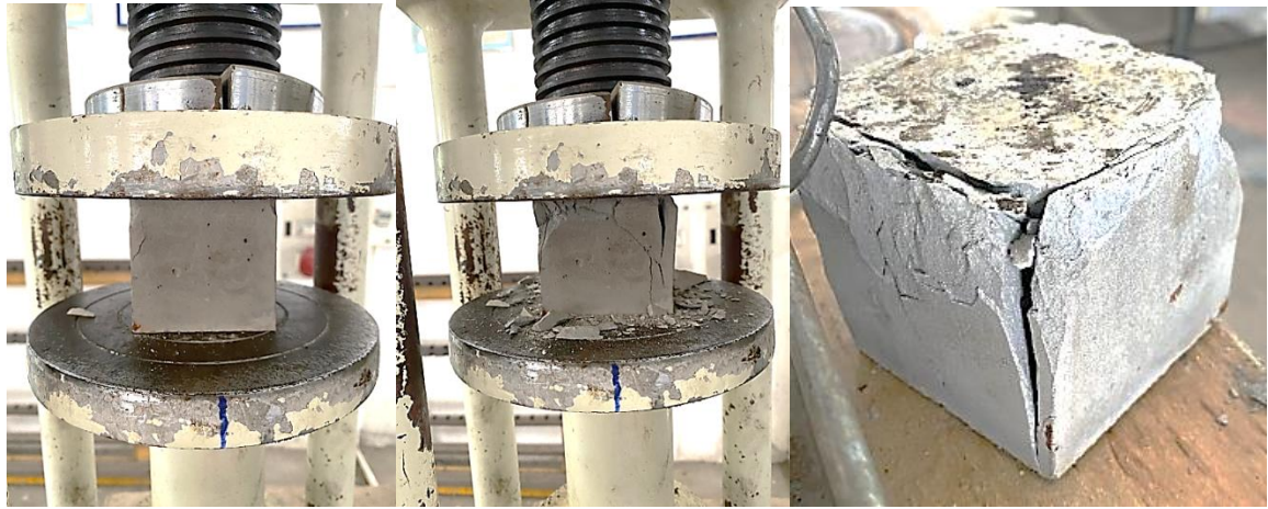
Figure.19 Compressive load is gradually applied until the cube fails.
