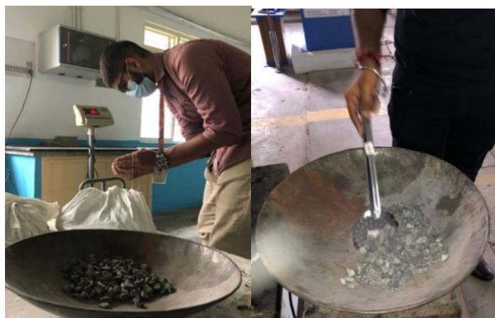
Figure.2 Aggregates weighed and graded as per its gradation
