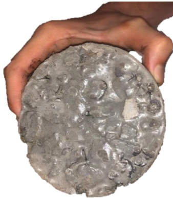
Figure.14 Sample specimen is extracted from the mould after 24 hours. Top view of the obtained CGBM sample is shown.
