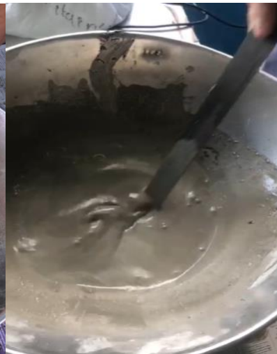
Figure.11 Gradual addition of water to obtain slurry
