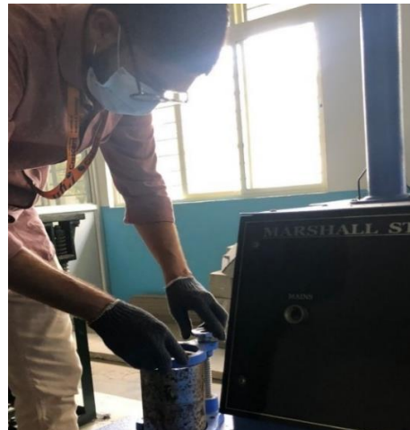
Figure.5 The hot bituminous mix is transferred to a Marshall mould (fitted with base plate & collar), fixed using spring tension for compaction.
