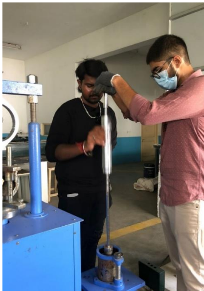
Figure.6 Compaction of mould to obtain a test specimen. It can be given 50-75 blows depending on rate of compaction.
