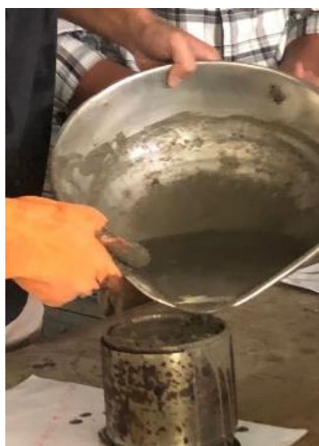
Figure.12 Mould is inverted (after removing base plate) and grout is poured.
