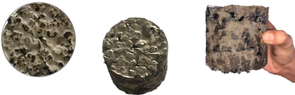
Figure.18 Grout with desirable proportion of water and cement (w/c ratio = 0.55) showed full depth penetration and adequate strength.
