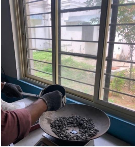
Figure.4 Melted bitumen is then poured into the mix. Trials are performed for different bitumen contents (%).
