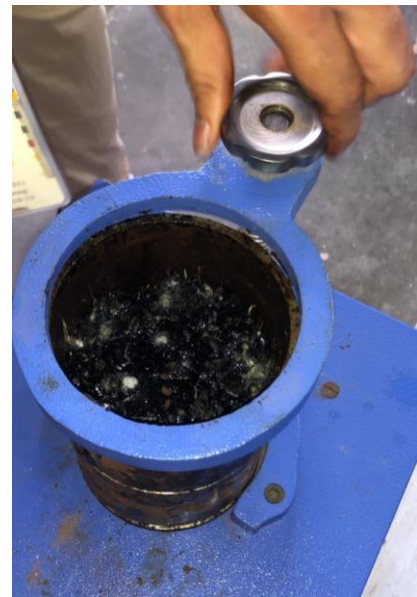
Figure.7 For Premix carpet, compaction is done on both sides, mould is removed and then kept for cooling.
