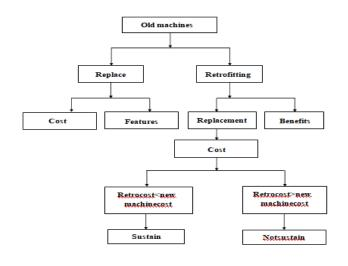
As our study on retrofitting we have done in our workshop. We decided to retrofit the old machine by changing some of the parts. So we list out the parts which can be retrofitted and then decided which part of machine is essential to retrofit. We had some machines which were rarely used due to the work done by other machines, so these were only occupying space .So the company decided to retrofit some parts of these machines and make it able to work efficiently. [3]
