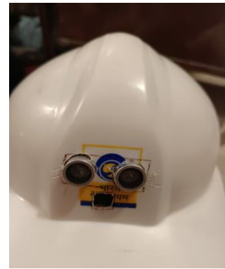
Fig. 2. Ultrasonic Sensor and Camera on Smart Hat
