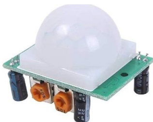
Fig. 7. PIR Motion Sensor
