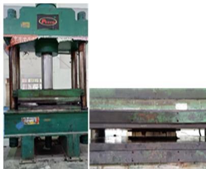
Fig. 2f Placing Steel Mould In Press
