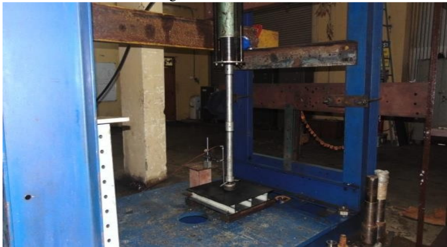
Fig. 3. Test Rig For Bending Load Test
