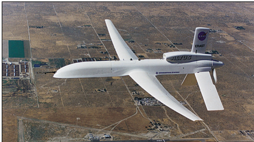
Figure 10. Prototype of High Altitude Aircraft Altus Fuel Powered UAV – Source: General Atomic
