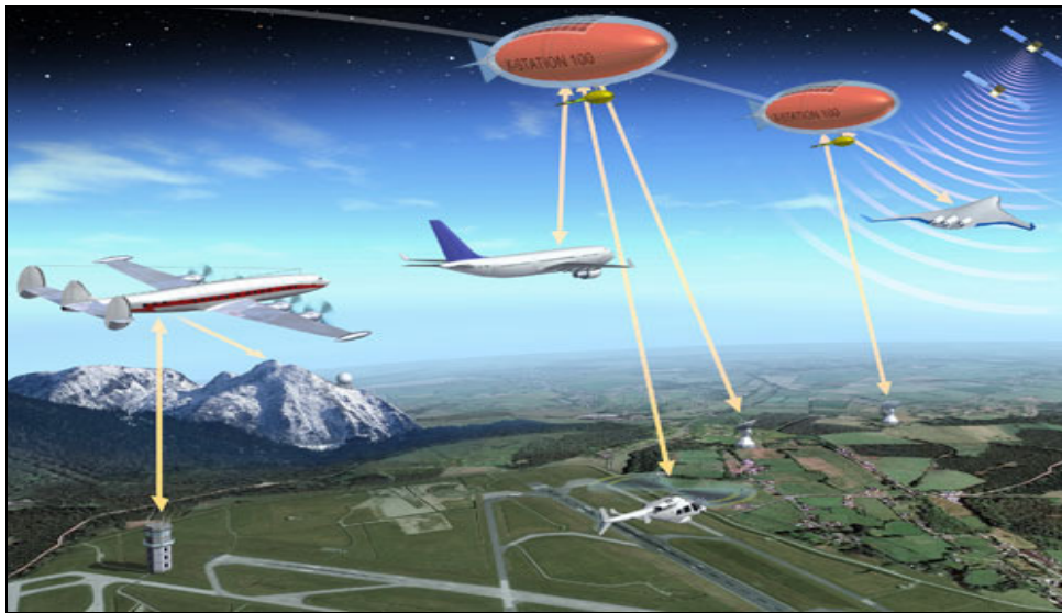
Figure 17. Hypothetical SPS Network for Aeronautical Communications – Sources: Ilcev
