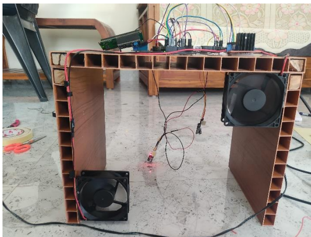
Fig 5: Implementation for two layer Oliver Ridley egg incubation.
