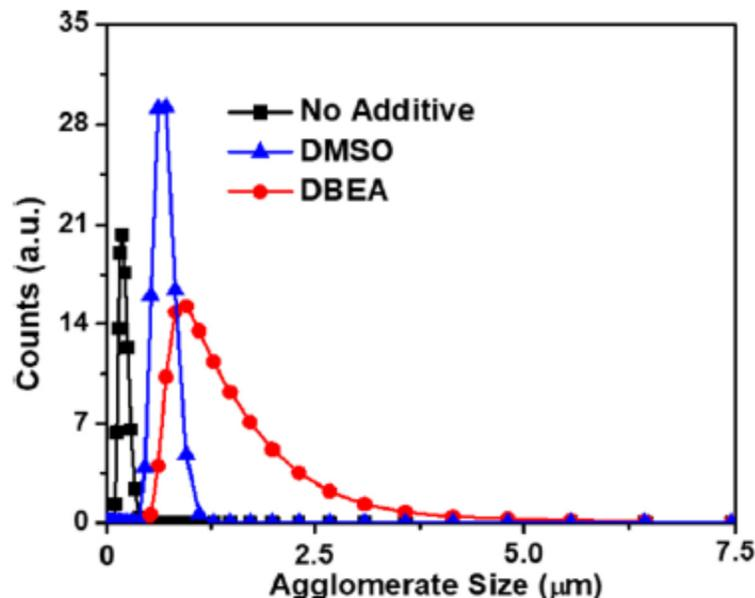
**Fig. 5.  $\text{PbI}_2$ -DBEA-MAI and  $\text{PbI}_2$ -DMSO- MAI adduct clusters size distribution in precursor solutions in comparison to a pristine device without any additive.**
