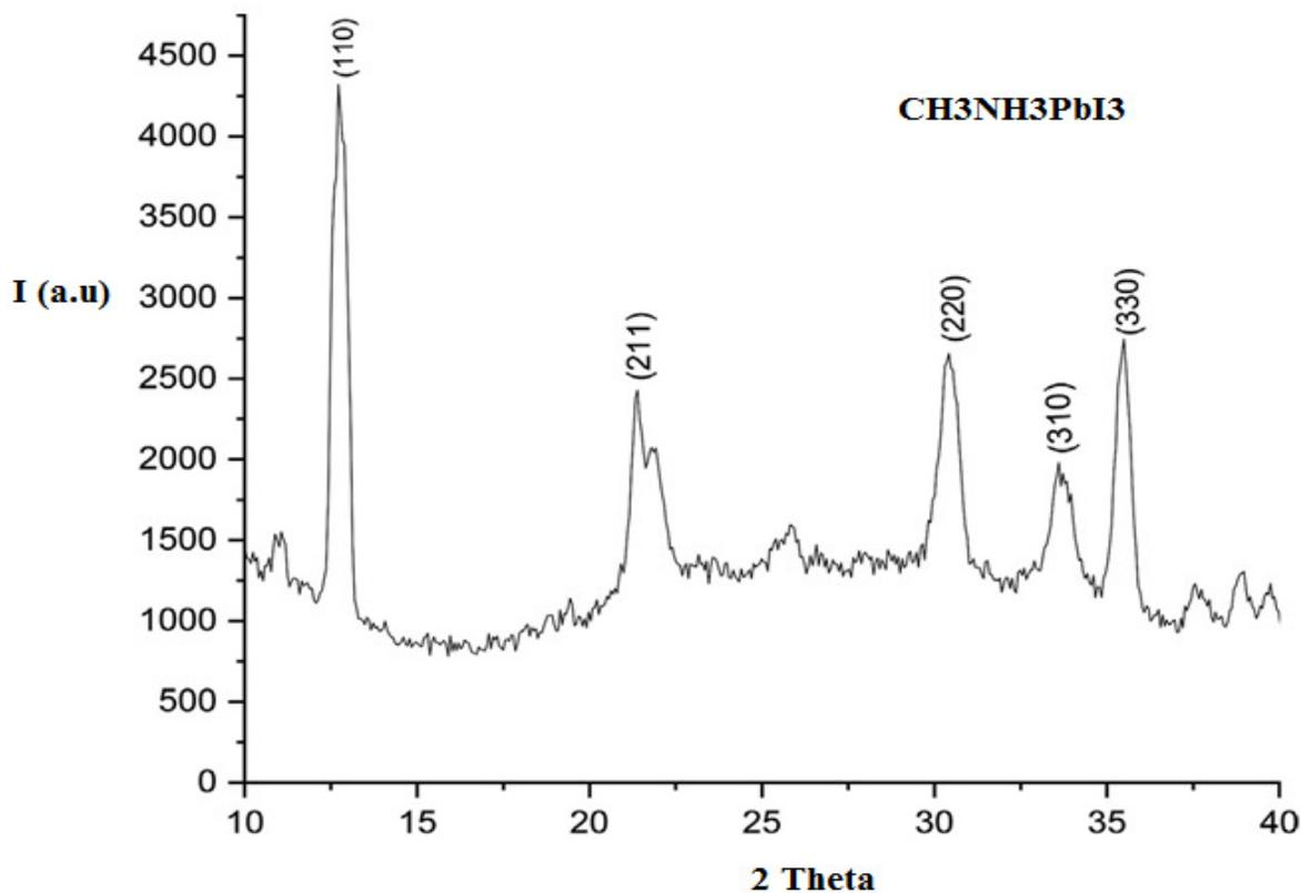
**Fig. 1. X-ray diffraction (XRD) of  $\text{CH}_3\text{NH}_3\text{PbI}_3$  perovskite**
