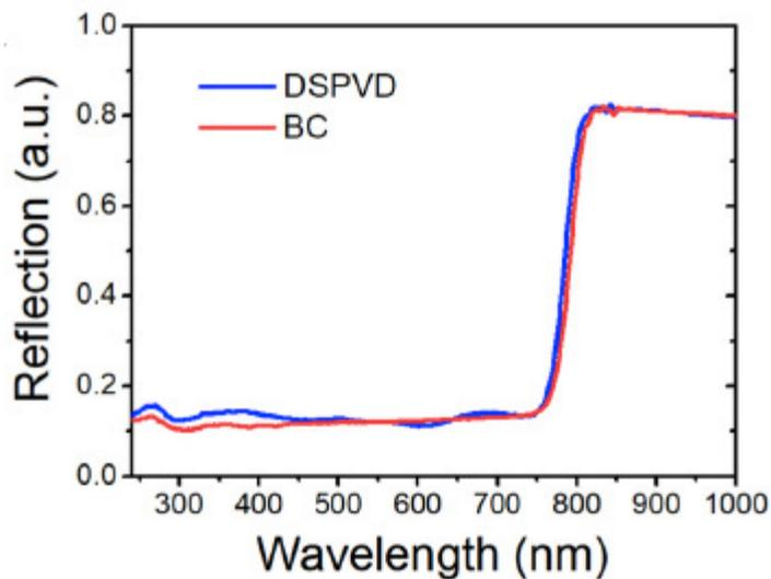
**Fig.4.** UV-Vis diffuses reflectance spectrum MAPbI<sub>3</sub> perovskite films.
