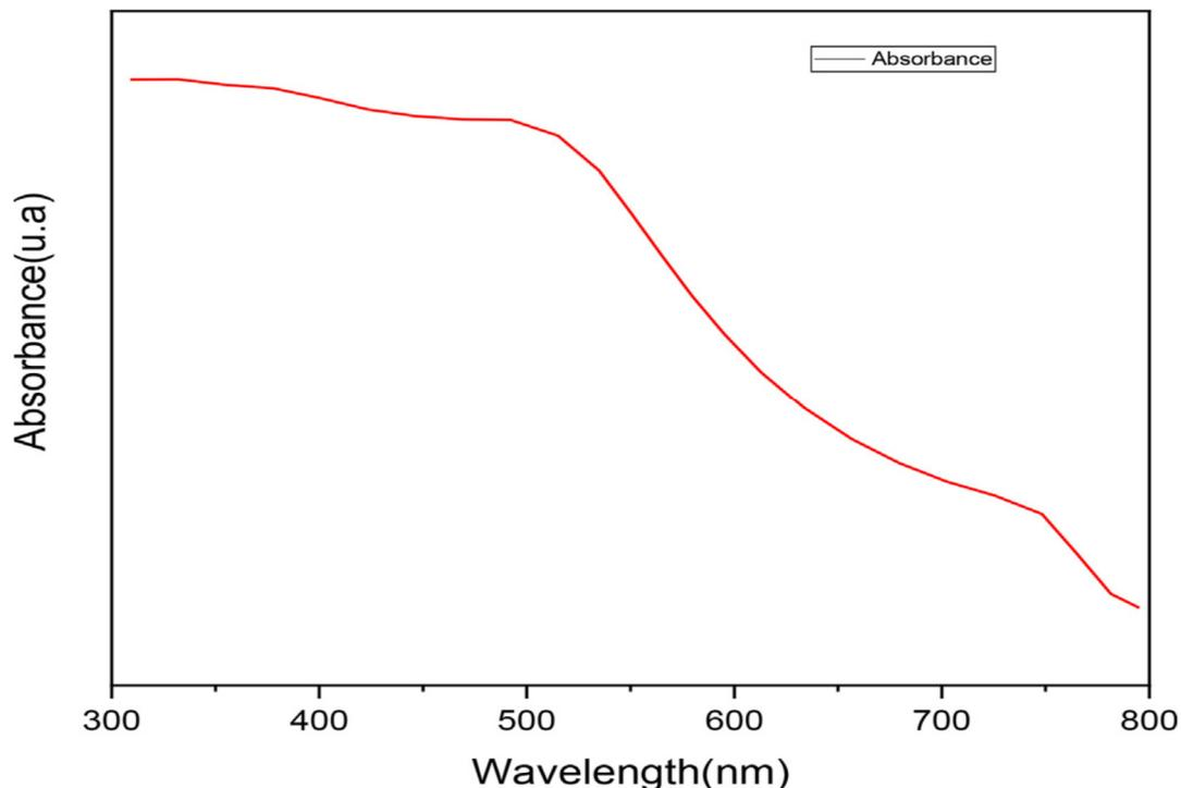
**Fig. 2. Optical absorbance spectrum of CH<sub>3</sub>NH<sub>3</sub>PbI<sub>3</sub>**
