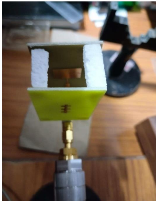
Figure 4: Fabricated Antenna setup with Vector Network Analyzer
