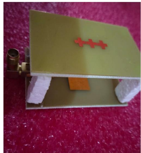
Figure 3: Fabricated 3x1 Metasurface Antenna (a) Top View (b) Side View
