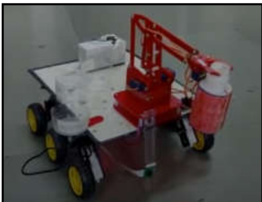
Fig3 Voice controlled Prototype Robot System Fig4 Image processing initiated and Robot picking metal
