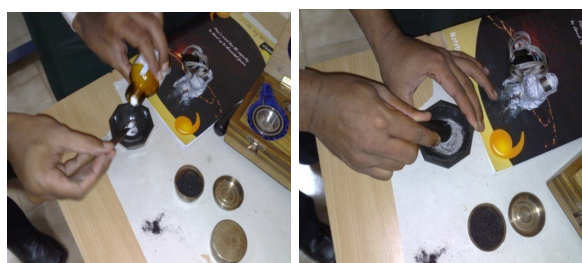
Figure 4.4: Preparation of Sample for FTIR Scan
