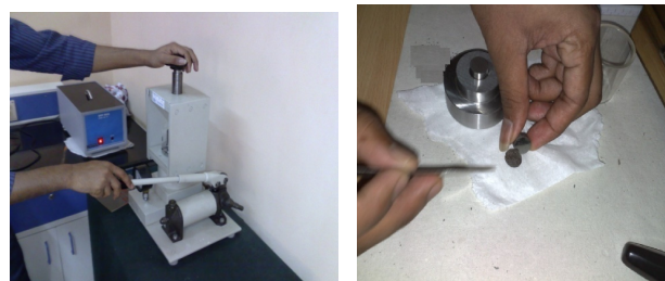
Figure 4.5 Pelleting the Sample
