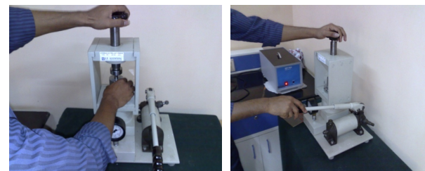
Figure 4.4: Preparation of Sample for FTIR Scan
