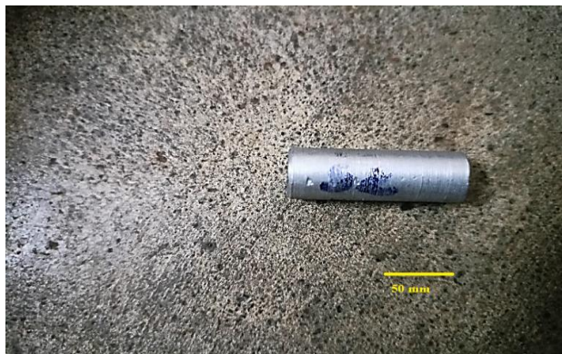
Figure 4. Experimental specimen after the wear test sample 2
