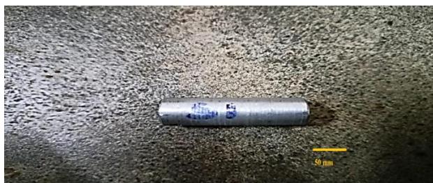
Figure 3. Experimental specimen after the wear test sample 1
