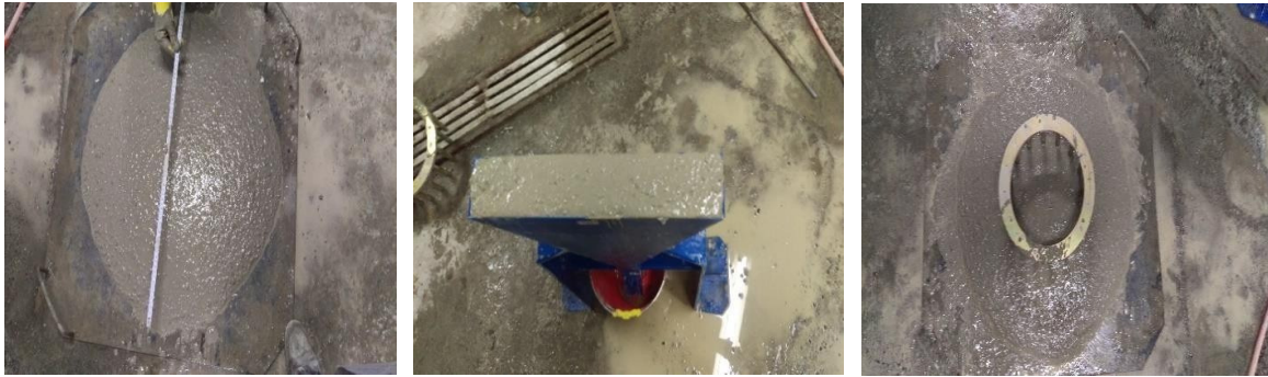
Fig. 2. Rheological tests set up for determining the flow ability and passing ability of mixtures.
