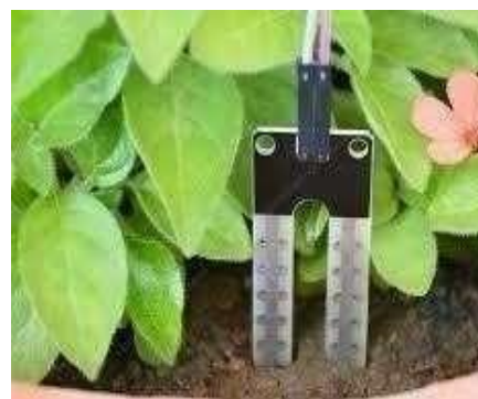
Fig :4.2 Soilmoisture sensor
