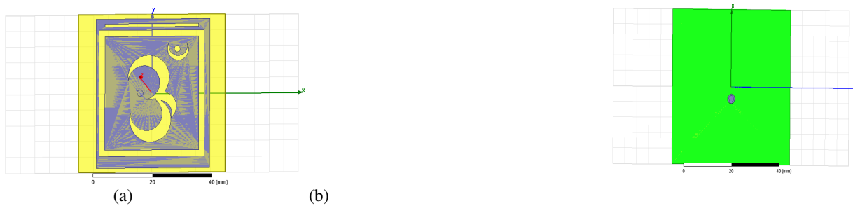
Fig 2: Microstrip patch antenna with no defected ground (a) Top view of antenna (b) bottom view of antenna
