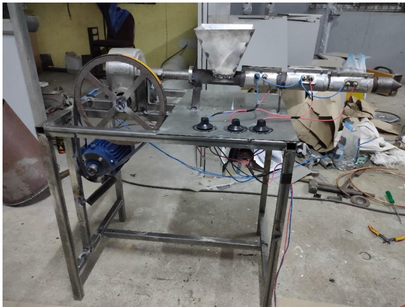
Fig. 9 . Fabricated model of plastic recycling by injection moulding 3D printer filament Setup
