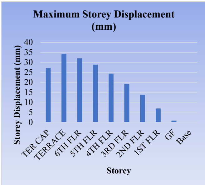
Graph1.6: Maximum Storey Displacement of Earthquake Zone-5
